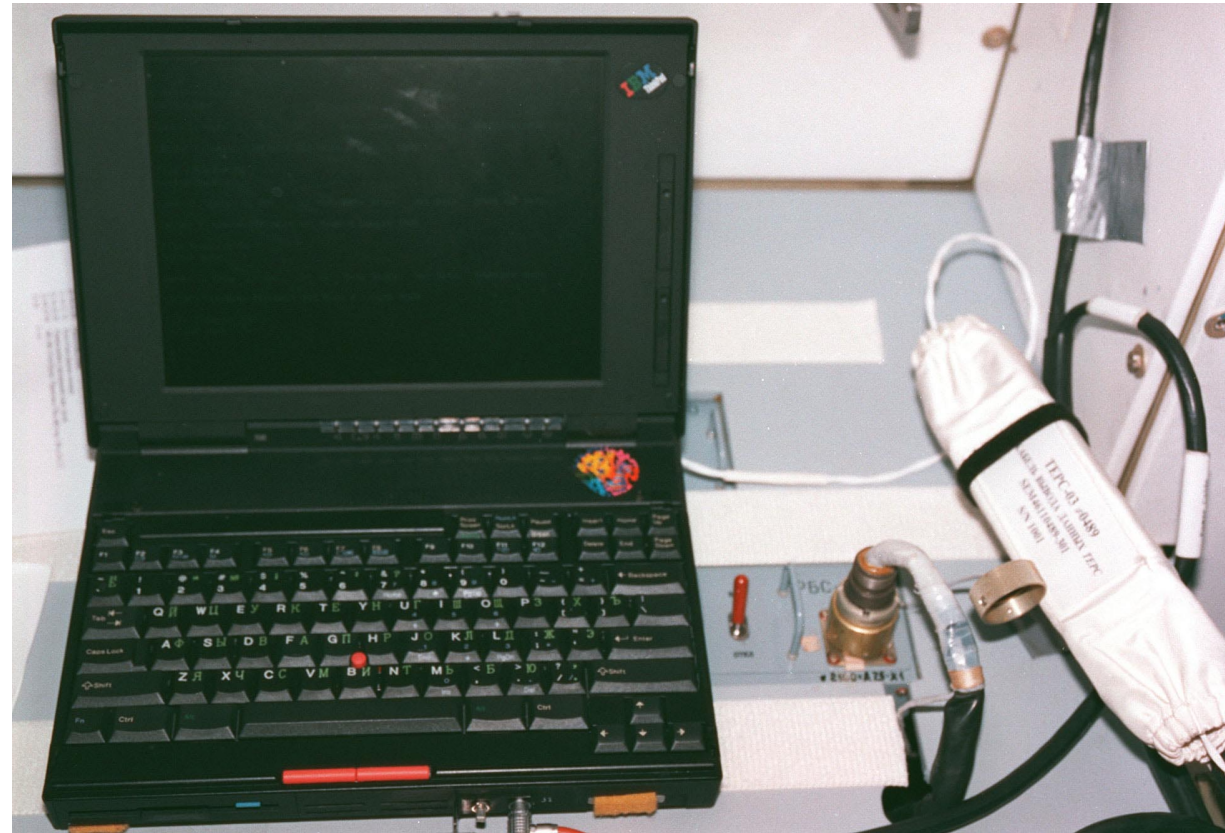
Figure SMP-135 TEPC Cable Connected to the MIPS-2L Near an RBS NM22-190-20
